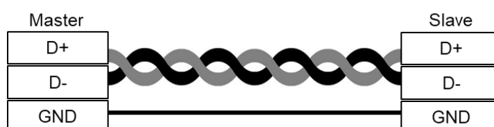
RS-485 2-wire cable (Twisted Pair)
