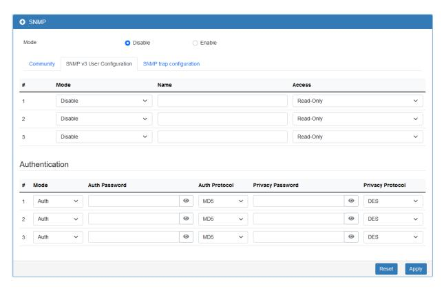
For SNMP v3 User Configuration, you need to register authentication and allow a receiver that confirm the packet was not modified in transit. There are three options to set up SNMP v3 Configuration.
