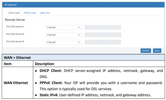
When selecting "DHCP Client", you can set up DNS Server Configuration.
