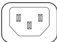
The 850X-28 can automatically adjust the AC power setting to adapt to any voltage supply in the range 100~240 VAC 50/60Hz. Connect the one end of the supplied AC power cord to the AC power connector on the rear panel and the other end into a properly grounded power outlet.
