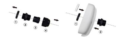
**STEP 4:** Put the Ethernet cable through the hole of the bottom cover and make a new RJ45 connector.
