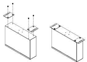
**STEP 2:** Use the screws to attach the bracket of the device for wall mounting.
