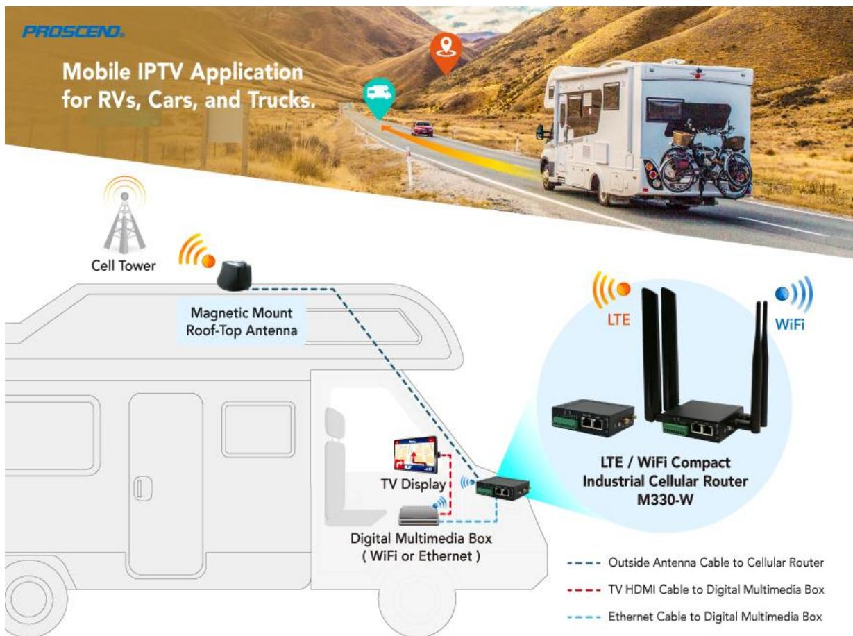
The 4G LTE WiFi Cellular Router M330-W with an outdoor 5-in-1 antenna enhances stable signal in IPTV application for RVs.
