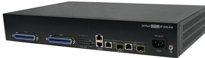
**Proscend 724M Series** is a 1.5U compact 24-port VDSL2 IP DSLAM with 2 Gigabit Ethernet Combo interfaces and built-in POTS splitter. It is compliant to ITU-T G.993.2 standard and supports VDSL2 30a profile that features 100Mbps of symmetric data rate over the existing copper wires. **724M Series** is an ideal choice for Carriers, ISPs and System Integrators that are looking for a high performance broadband solution for their triple play (Video, Voice and Data) applications.
