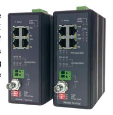
Under **Remote Power Mode**, each **101MP** is equipped with four 10/100Base-TX IEEE 802.3at PoE Ports for a total power budget of 30W; Support any remote IEEE 802.3at/af powered device (PD) like Wi-Fi Access Point, IP phone, and IP Camera. It enables centralized management of power supply from a single location for easy, efficient and cost-effective installation.
